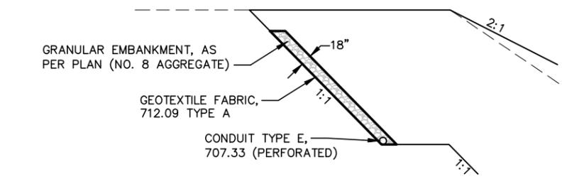
**BENCHING SLOPE DRAIN DETAIL**
