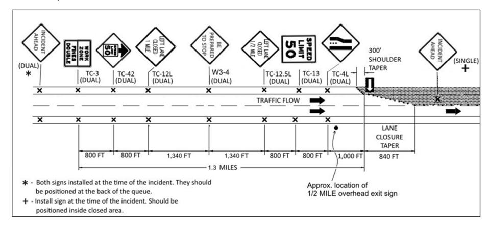
The following Temporary Traffic Control devices shall be used to affect a closure on a 3-lane section of the Ohio Turnpike if an incident is expected to last more than 24 hours.
