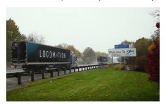
a truck platooning system to operate continuously through a multi-jurisdictional environment. The two-truck platoon traveled over 300 miles starting in Pittsburgh, across the Ohio Turnpike to Michigan. Trucks transported food between the Greater Pittsburgh Area Food Bank in Pennsylvania, the Toledo Northwest Ohio Food bank, and the Forgotten Harvest Food Rescue Organization in Michigan.
