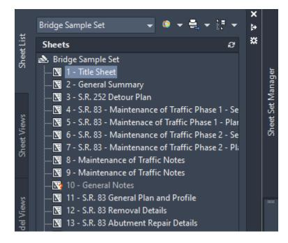
Maintaining the sheet set included in the example sheets provides the organizational structure and default settings for a new set of sheet plans. Specify that folders are created corresponding to the subset storage paths of the sheet set. After you create an empty sheet set with this option, you can Import layouts or create sheets individually.
