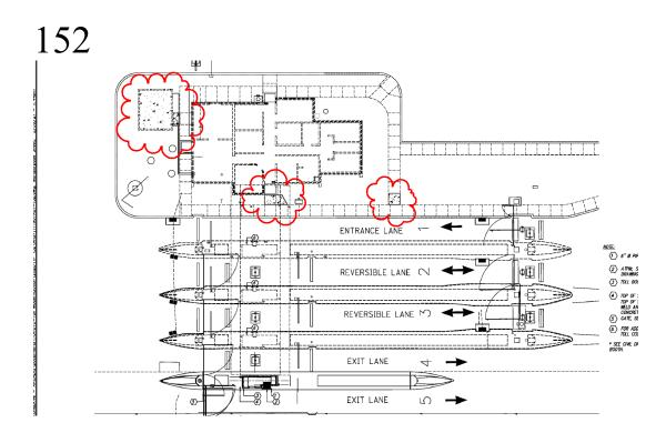
A#8 The sidewalk removal and replacement limits are shown on Plan Sheet A20 (C-11) for Toll Plaza 64 and Plan Sheet B18 (C-9) for Toll Plaza 152. It is not anticipated to remove and replace any sidewalk beyond what is shown on the referenced sheets.
